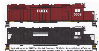
Typical Layout for FURX ex Norfolk Southern GP38-2's. It's mostly just a Paint out of the NS Scheme. At least 1 has been painted in the HLCX style Cornell Red Scheme. The 5509 has been rebuilt and it currently leased to the New Hampshire Northcoast.
